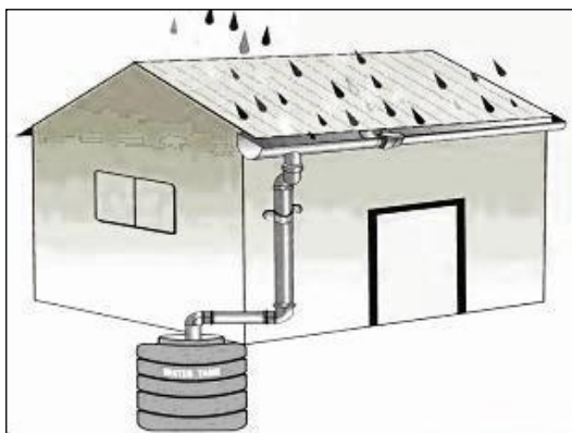
Fig. 3. Schematic Diagram of Roof Top Rainwater Harvesting
